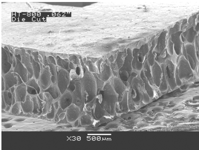
Fig. 8. BISCO HT-800 1.59mm Steel Rule Process
